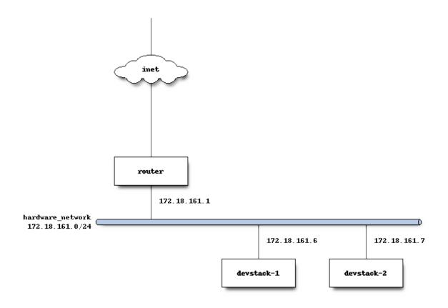
After DevStack installs and configures Neutron, traffic from guest VMs flows out of *devstack-2* (the compute node) and is encapsulated in a VXLAN tunnel back to *devstack-1* (the control node) where the L3 agent is running.
