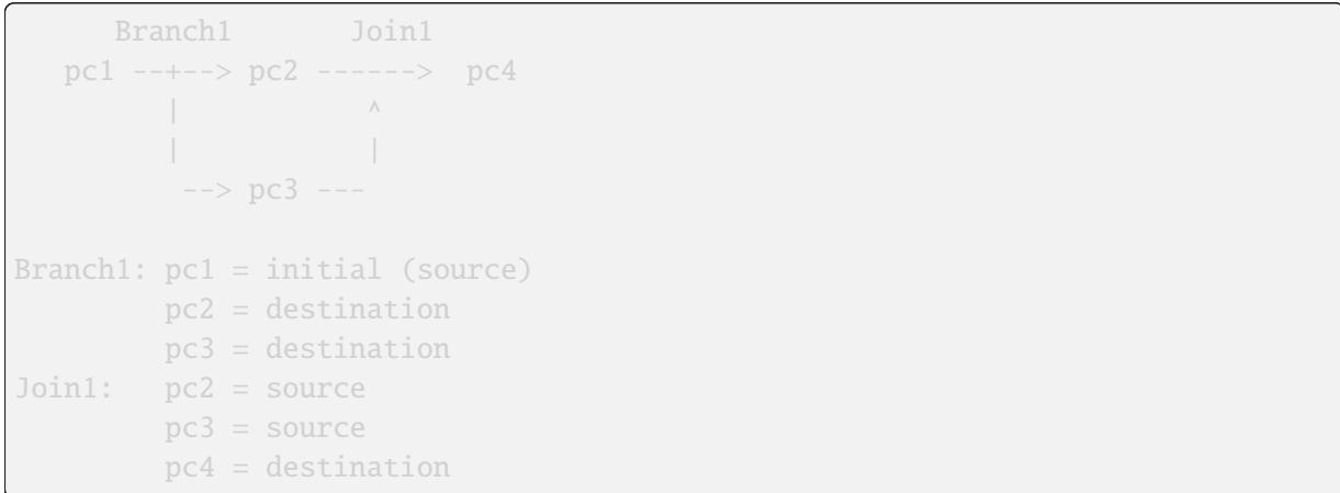
Since Port Chains resemble Service Function Paths, with the `chain_id` attribute mapping to a Service Path Identifier (SPI), they are used as the SFPs for the Service Graph, and consequently Service Graphs in networking-sfc allow the creation of dependencies between Port Chains (alongside traffic classification criteria, just like a normal Port Chain, via Flow Classifier).
