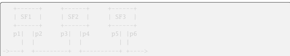
where p1 is the head of the Port Chain and p6 is the tail of the Port Chain, and SF1 has ports p1 and p2, SF2 has ports p3 and p4, and SF3 has ports p5 and p6.
