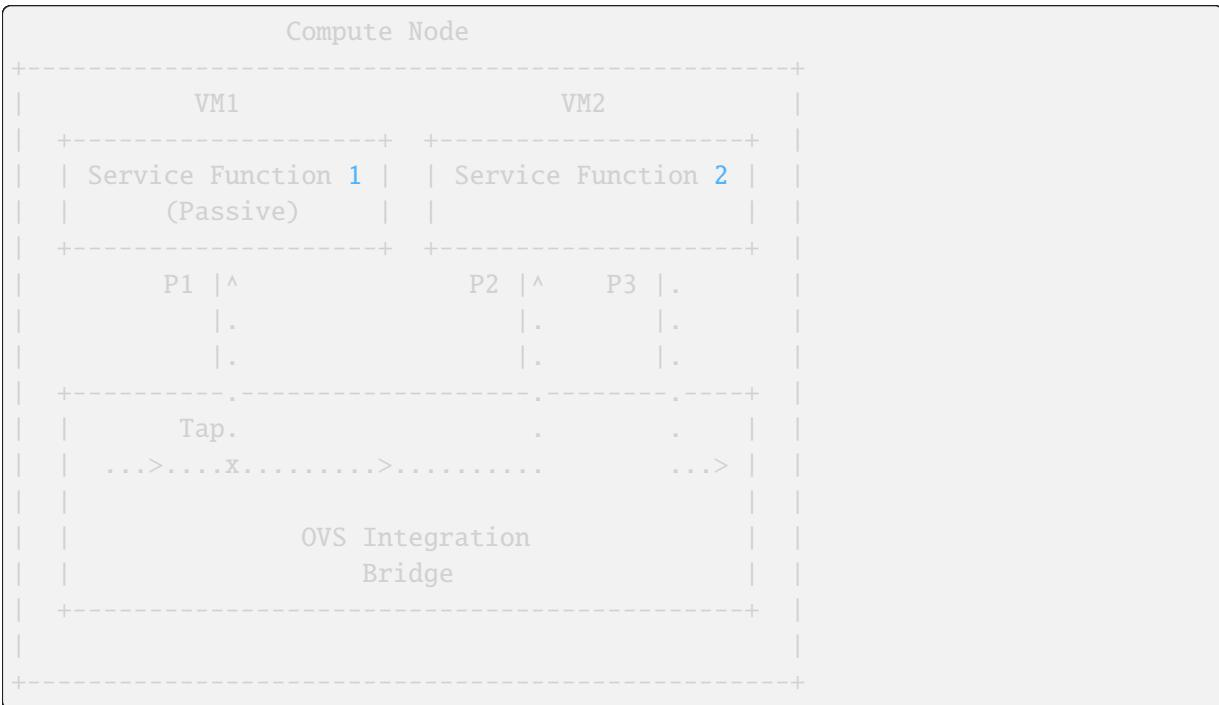
The tap will work regardless of whether the next hop SF is hosted on the same Compute node as the tap Port Pair as shown above or on another Compute node as shown below.
