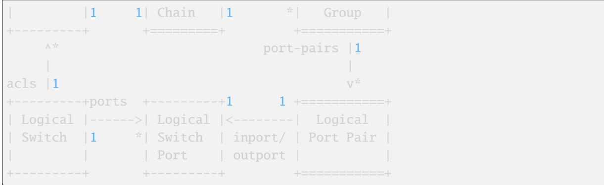
The OVN ACL actions are extended to include a SFC action with an `external_id` to reference the name of the Logical Port Chain (lchain) with which the ACL is associated. The `sfc` action means that the packet is allowed and steered into the port-chain.
